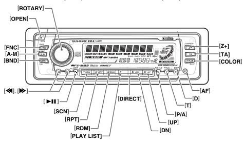
With the FLIP DOWN PANEL opened / Ouvrez le PANNEAU RABATTABLE ÖFFNUNG DER KLAPPSCHALTTAFEL / Apertura del PANNELLO APRIBILE Met het NEERKLAPBARE PANEEL geopend / Apertura del PANEL ABATIBLE DEN NEDFÄLLBARA PANELEN öppen / Abrindo o PAINEL RECLINÁVEL
